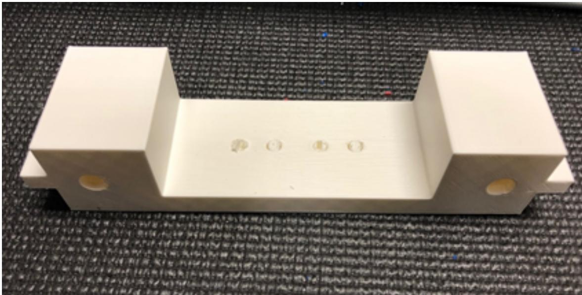
**Figure 30: Printed pickup bridge block (PLA).**
