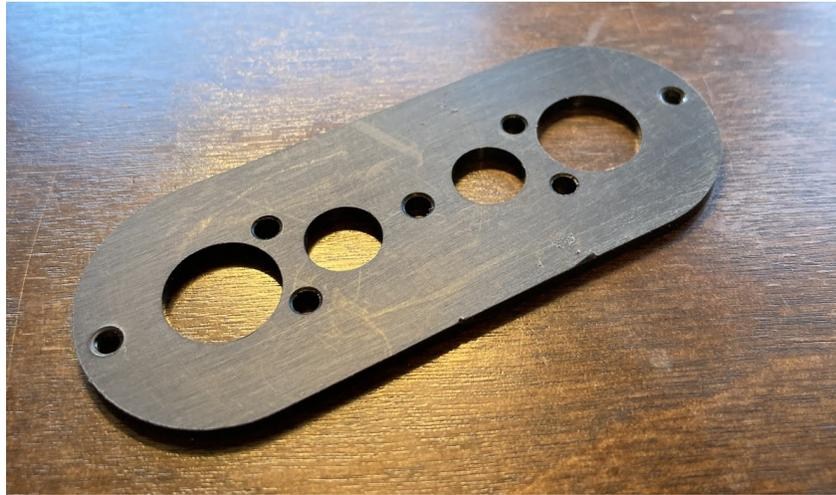
**Figure 22: Machined bobbin top plate (Delrin).**
