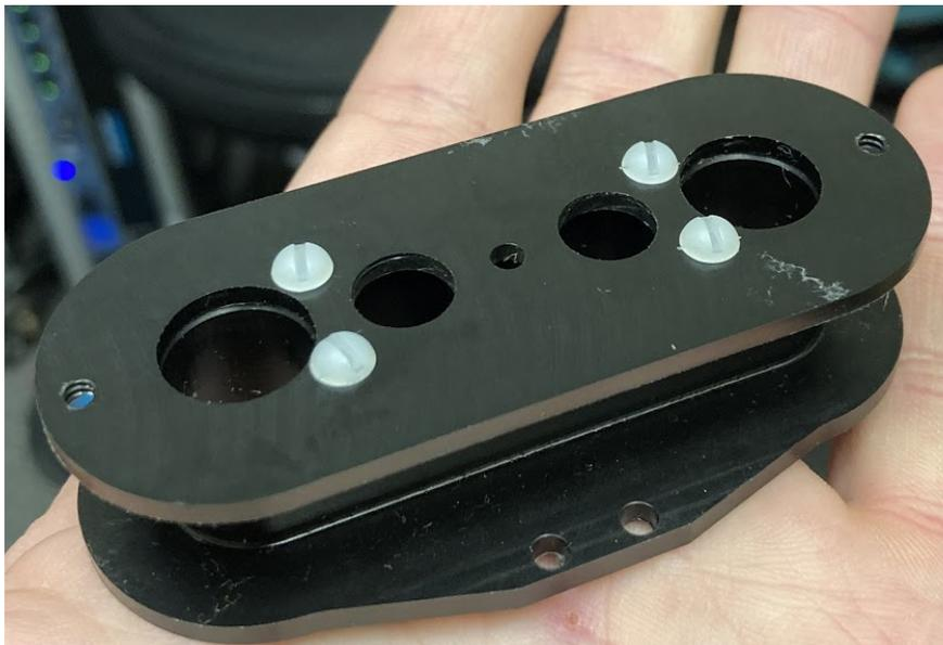
**Figure 32: Machined bobbin assembly.**
