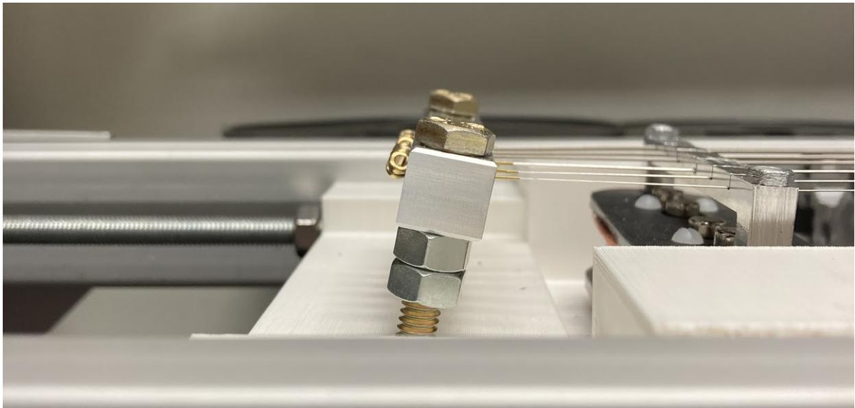
**Figure 53: Tailpiece bending as a result of testing.**
