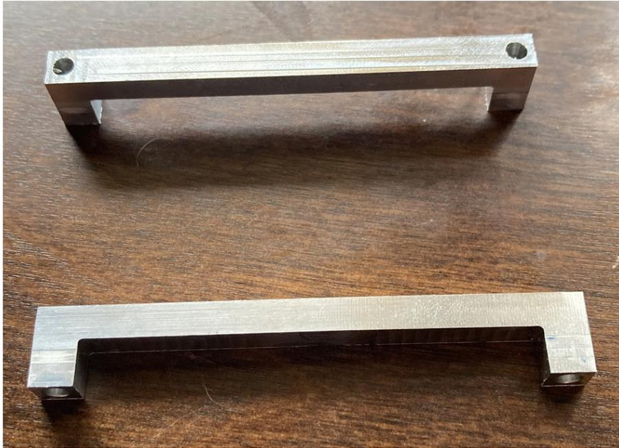
**Figure 24: Machined yoke profile (without wire EDM notches, aluminum).**
