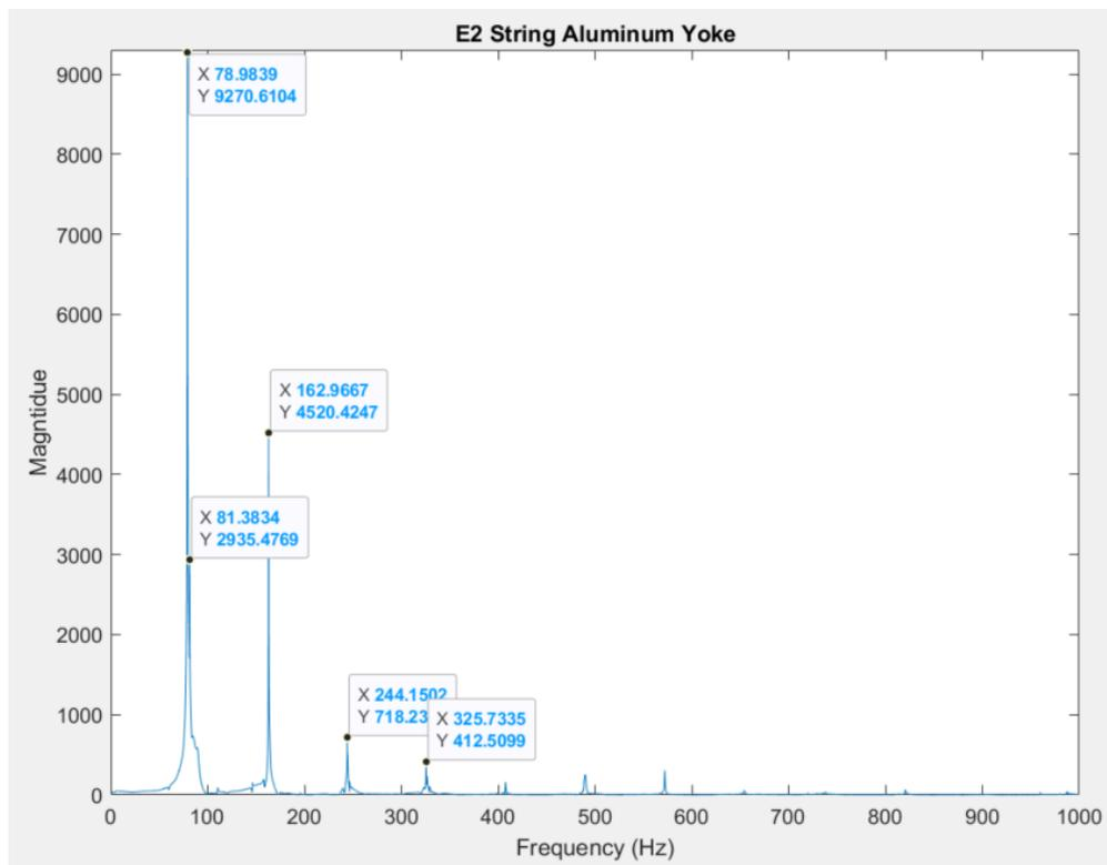
**Figure 41: E2 string (aluminum yoke, no bearings).**
