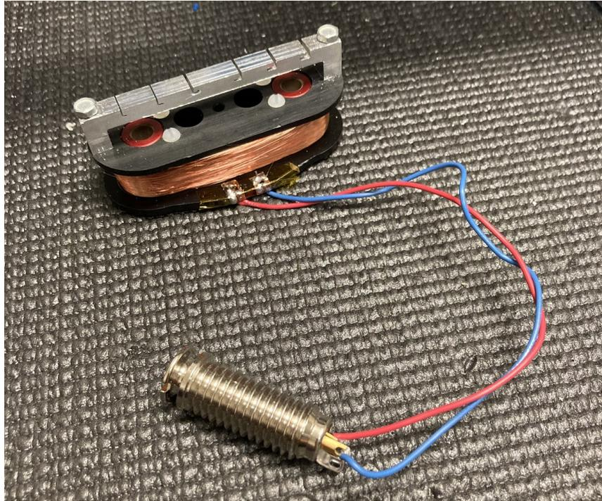
**Figure 35: Assembled pickup with bearings and aluminum yoke.**
