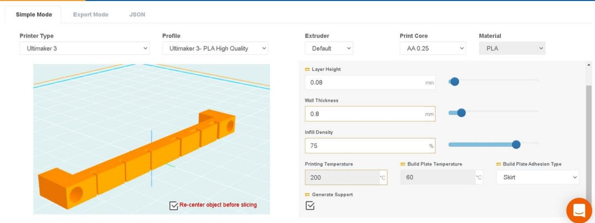
**Figure 26: Capture of how the printer settings are selected in 3DPrinterOS.**
