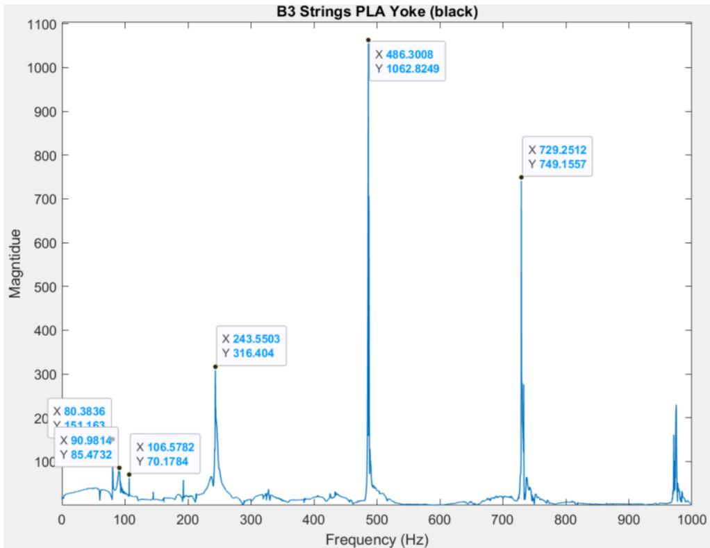
**Figure 51: B3 strings (PLA yoke, no bearings).**
