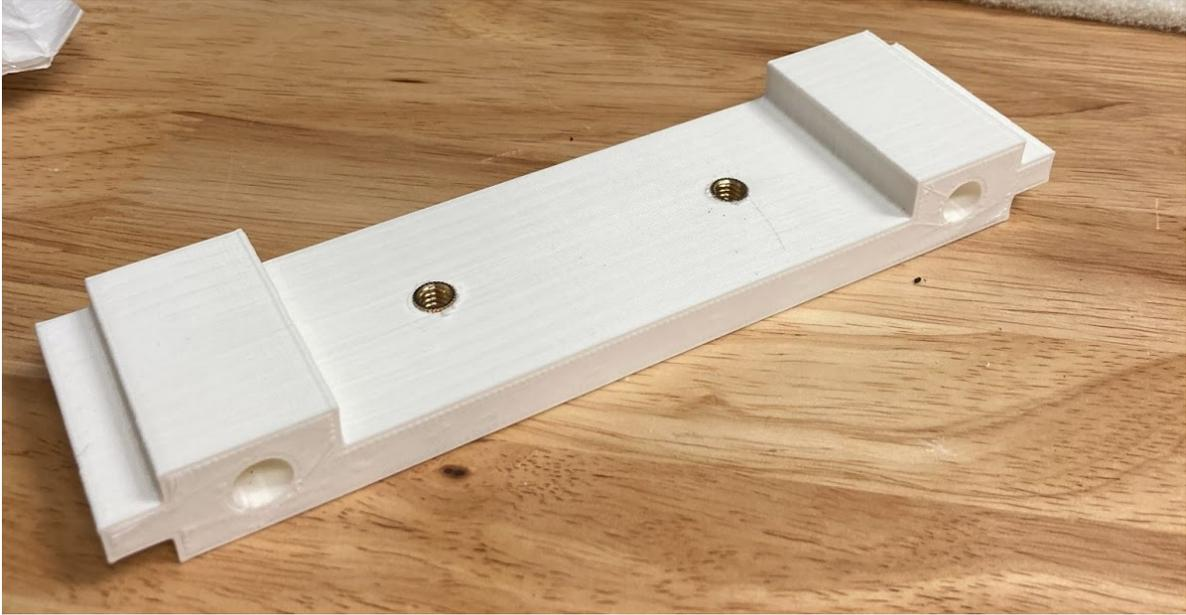
**Figure 31: Printed tailpiece bridge block with threaded inserts (PLA).**
