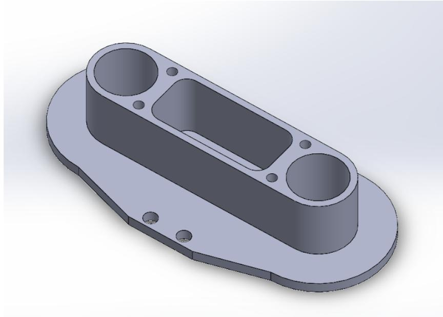
**Figure 10: Bobbin bottom piece 3D model.**
