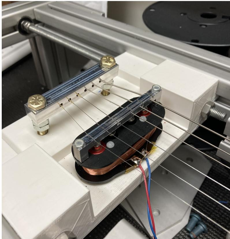
**Figure 37: Pickup and tailpiece setup on test rig**
