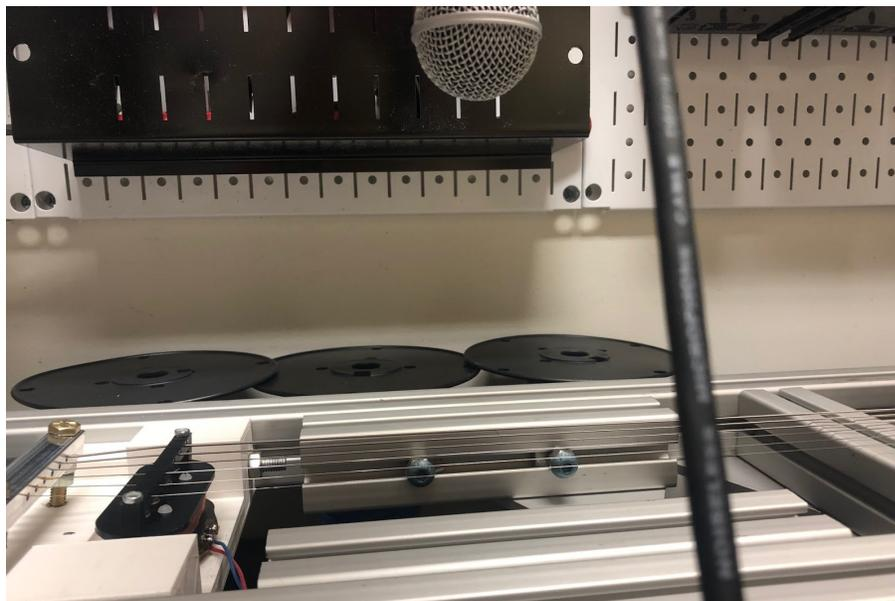
**Figure 40: Microphone placement for acoustic response.**
