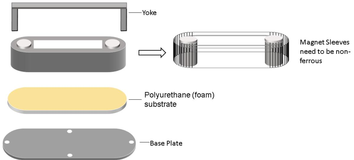
**Figure 5: Early layout of bobbin components.**
