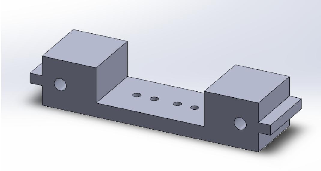
**Figure 19: Pickup bridge block for guitar component test rig.**
