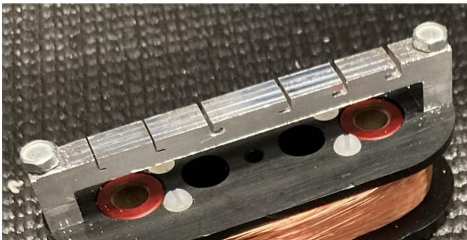
**Figure 25: Machined yoke (aluminum) fastened to pickup.**
