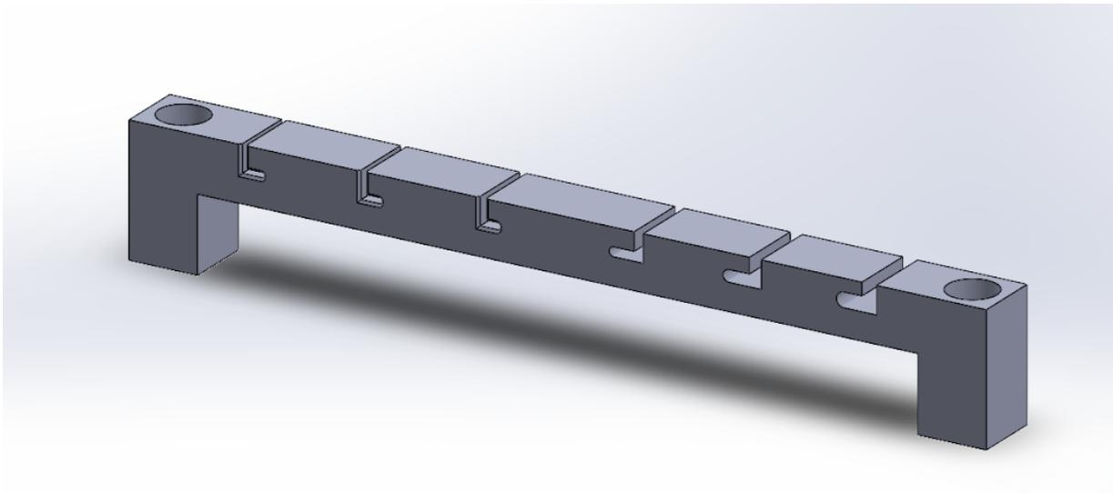
**Figure 14: Yoke 3D model with chamfers on three smallest grooves (for printing).**
