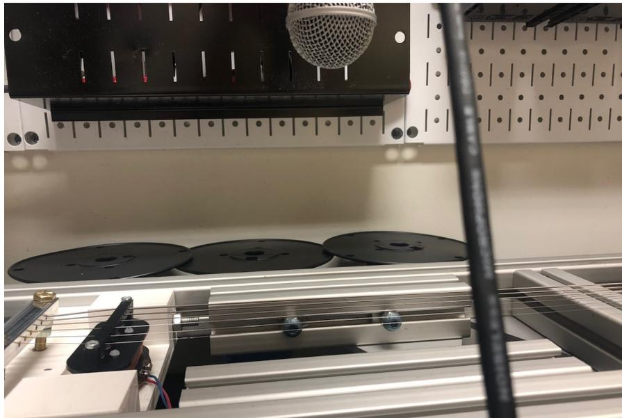
**Figure 40: Microphone placement for acoustic response.**
