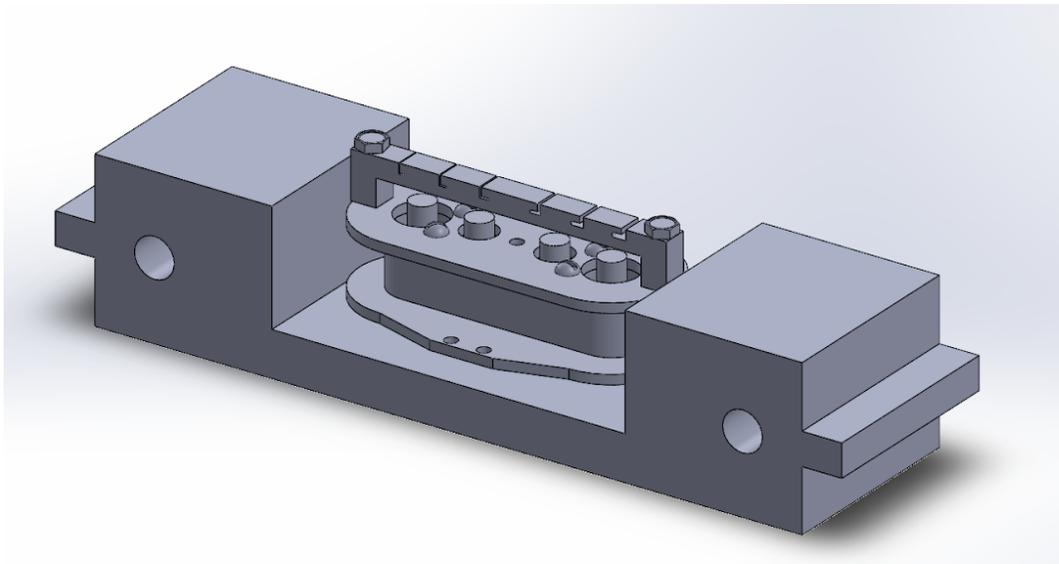
**Figure 20: Pickup bridge block and pickup assembly with magnets.**
