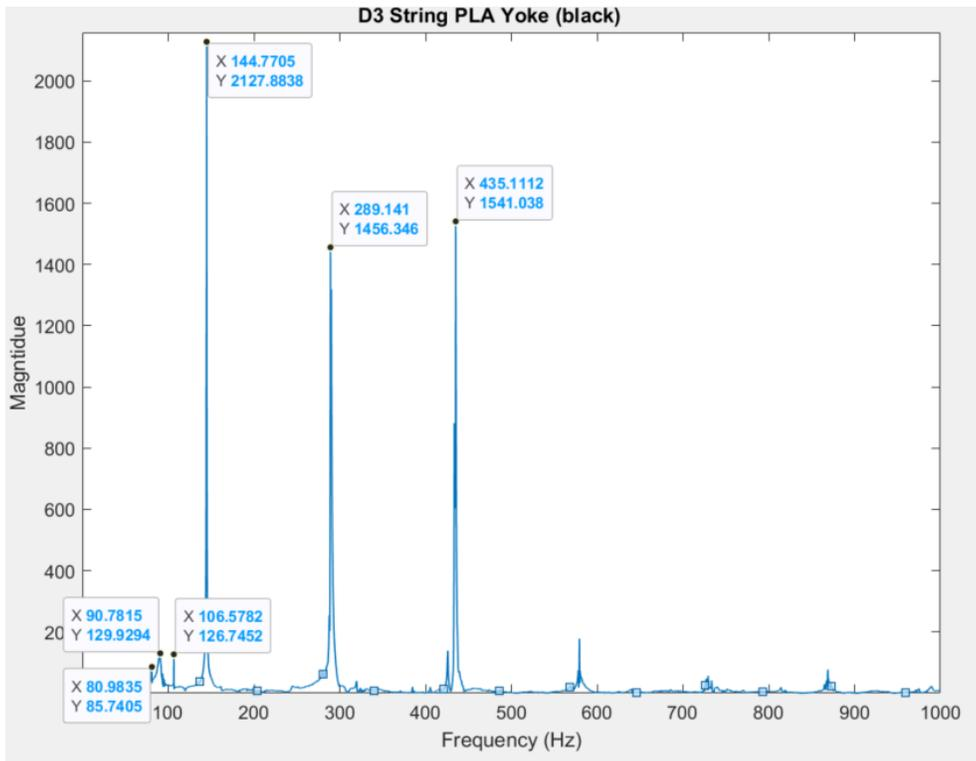
**Figure 49: D3 string (PLA yoke, no bearings).**
