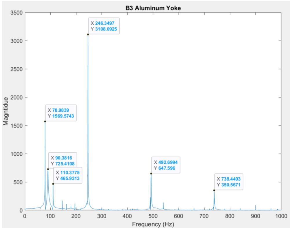
**Figure 45: B3 string (aluminum yoke, no bearings).**
