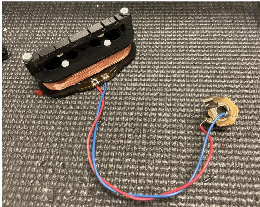
**Figure 36: Assembled pickup with PLA yoke, no bearings**
