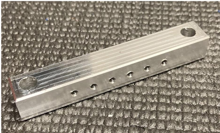
**Figure 23: Machined tailpiece (aluminum).**
