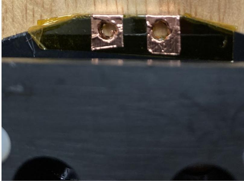
**Figure 33: “Sandwich method” for soldering coil leads.**
