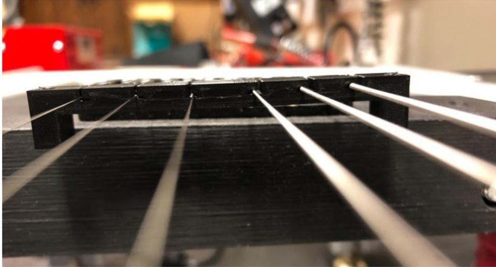
**Figure 29: Printed yoke (PLA) with chamfers.**
