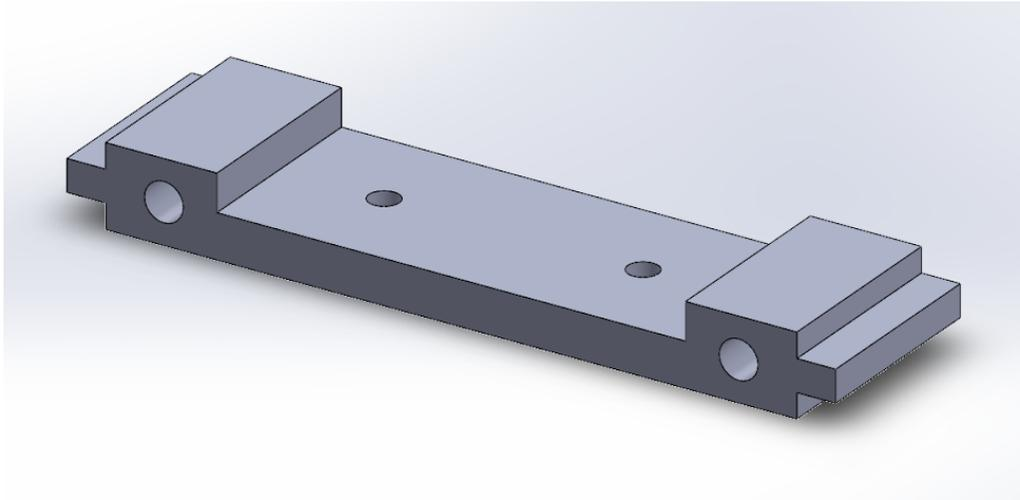
**Figure 17: Tailpiece bridge block for guitar component test rig.**
