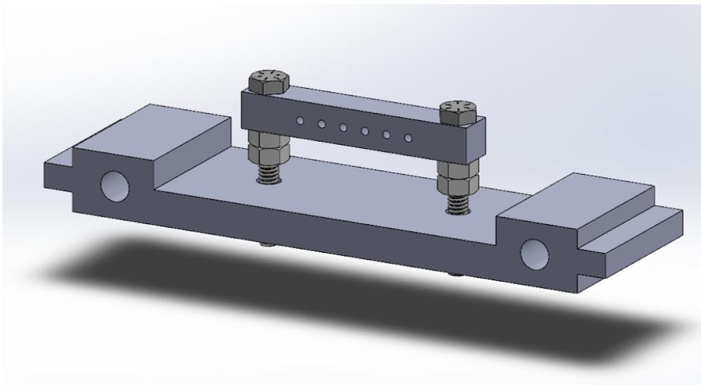
**Figure 18: Tailpiece bridge block with tailpiece and threaded bolts.**
