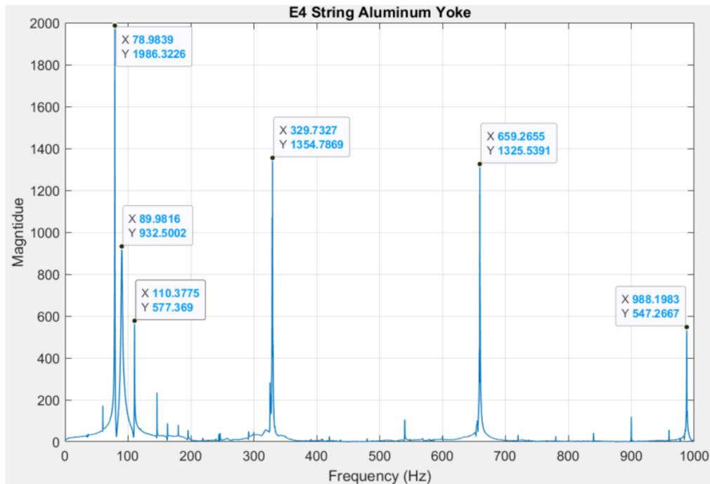
**Figure 46: E4 string (aluminum yoke, no bearings).**
