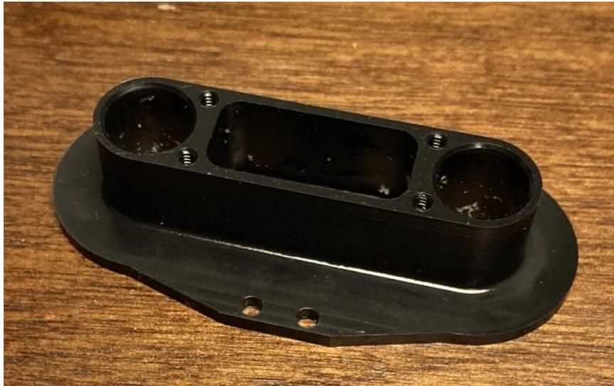
**Figure 21: Machined bobbin bottom piece (Delrin).**
