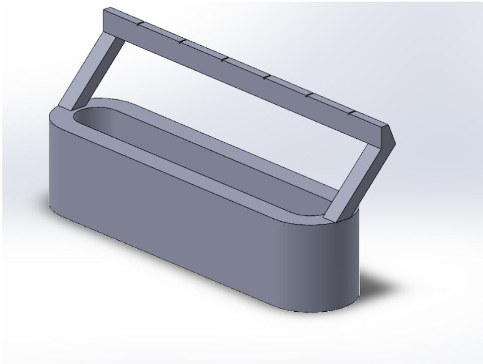
**Figure 1: Initial design 1 with notches for strings.**
