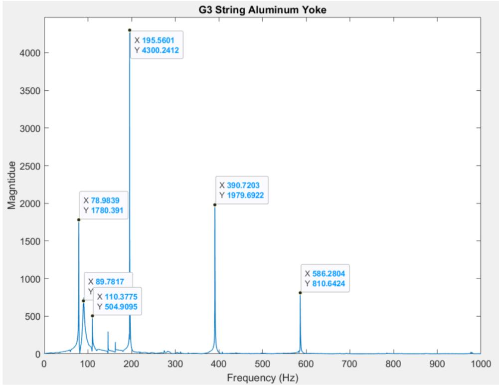
**Figure 44: G3 string (aluminum yoke, no bearings).**
