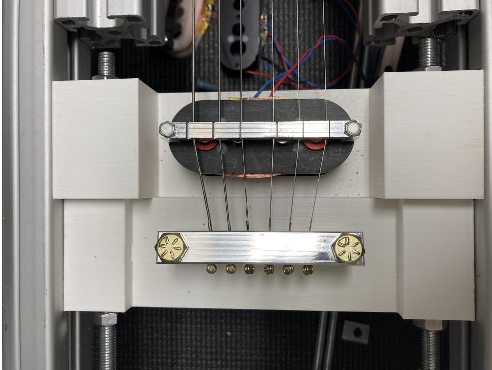
**Figure 38: Bird's eye view of pickup on test rig.**
