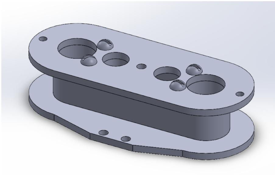
**Figure 12: Bobbin assembly 3D model.**
