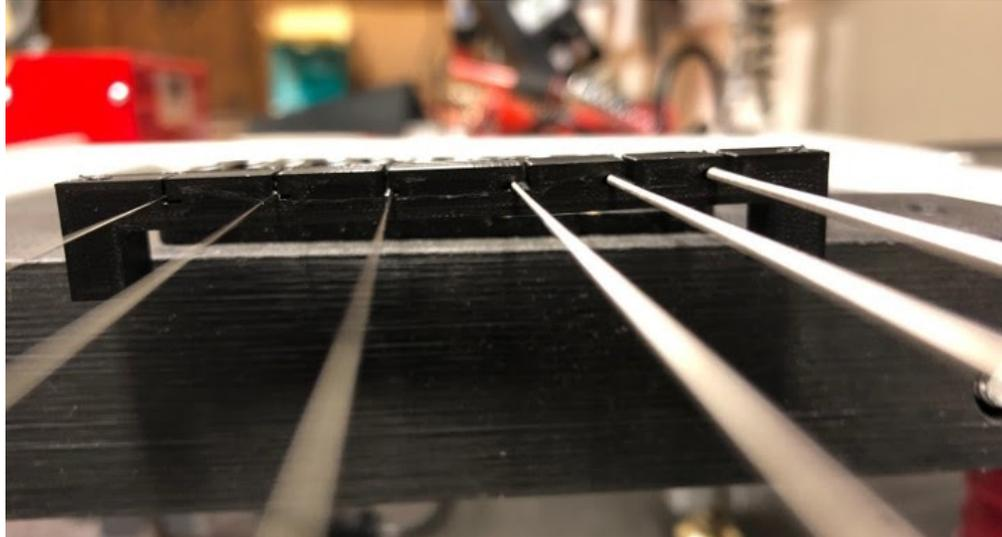
**Figure 29: Printed yoke (PLA) with chamfers.**
