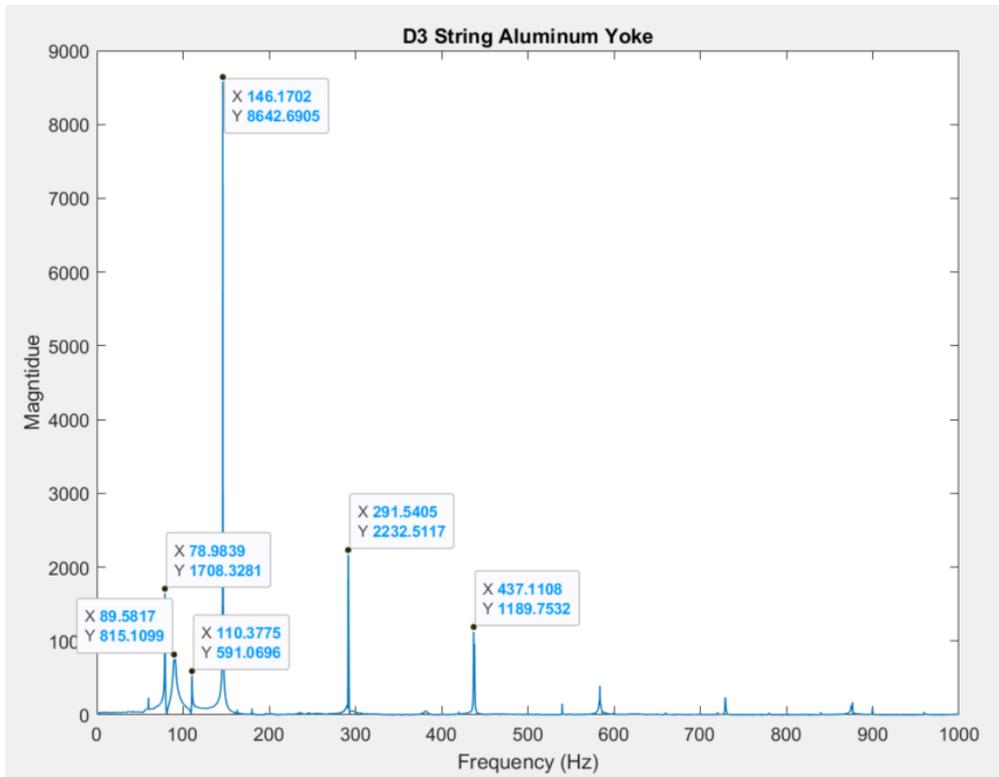
**Figure 43: D3 string (aluminum yoke, no bearings).**
