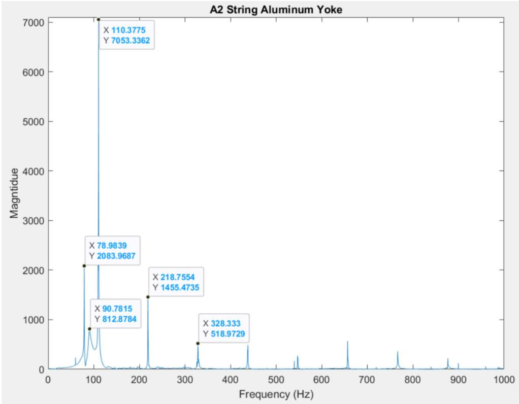
**Figure 42: A2 string (aluminum yoke, no bearings).**
