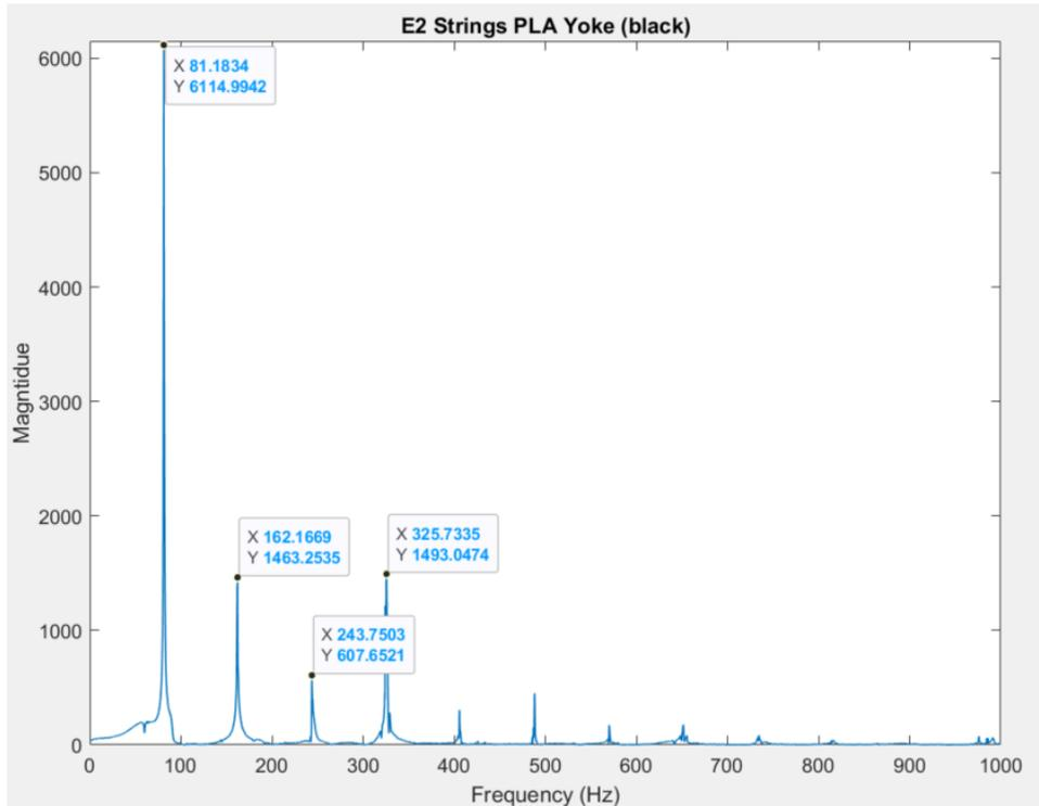
**Figure 47: E2 strings (PLA yoke, no bearings).**
