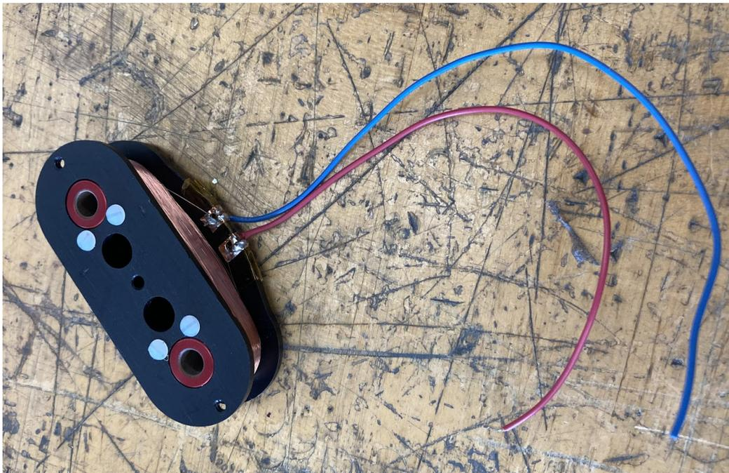
**Figure 34: Pickup with bearings (no yoke).**
