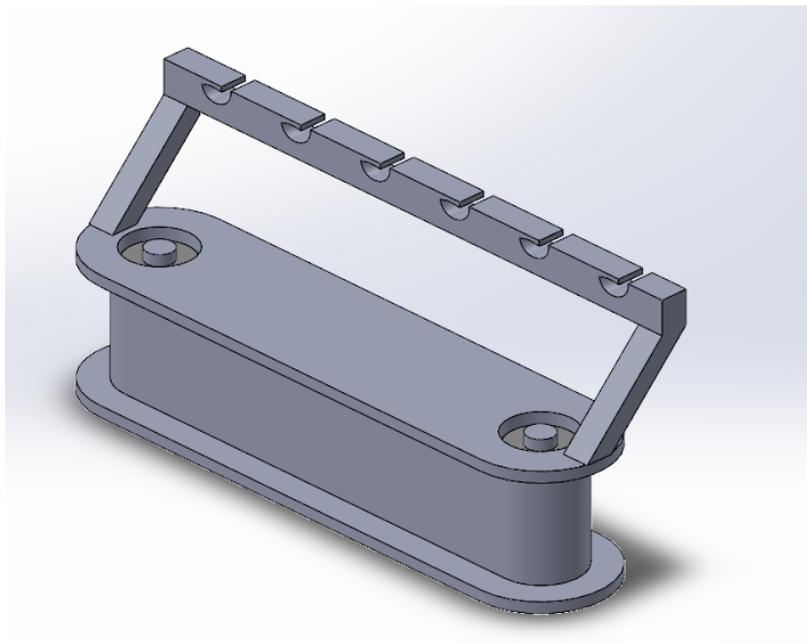
**Figure 3: Bearing concept for magnets to prevent side-to-side motion.**
