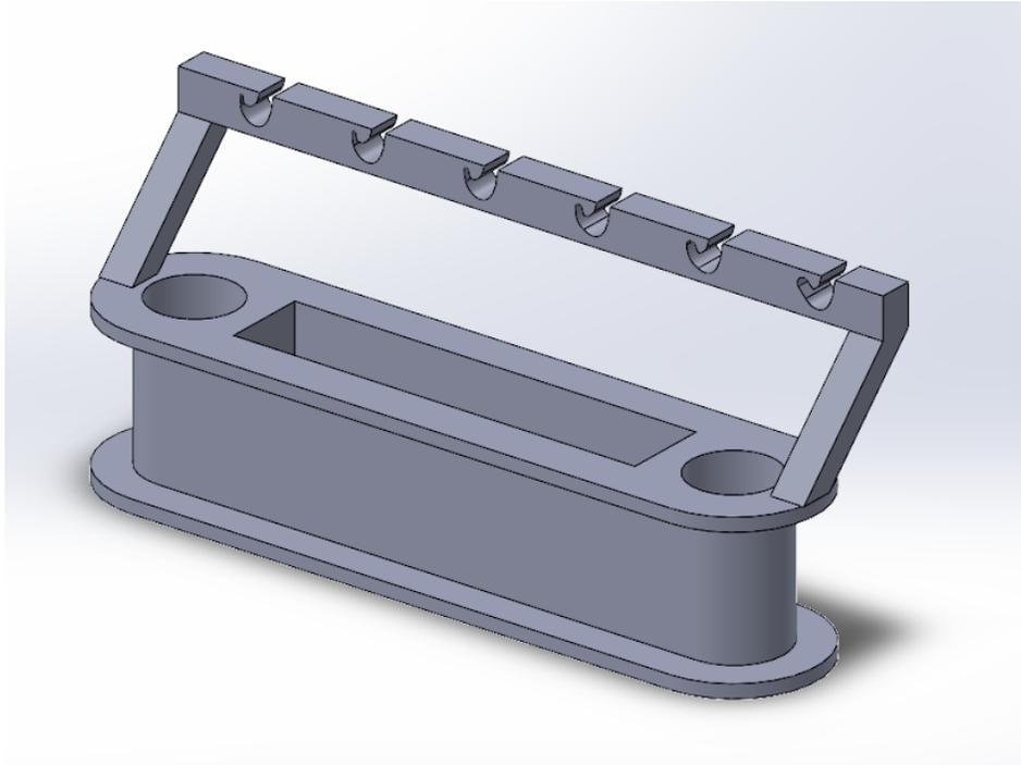
**Figure 4: Reduced material bobbin.**
