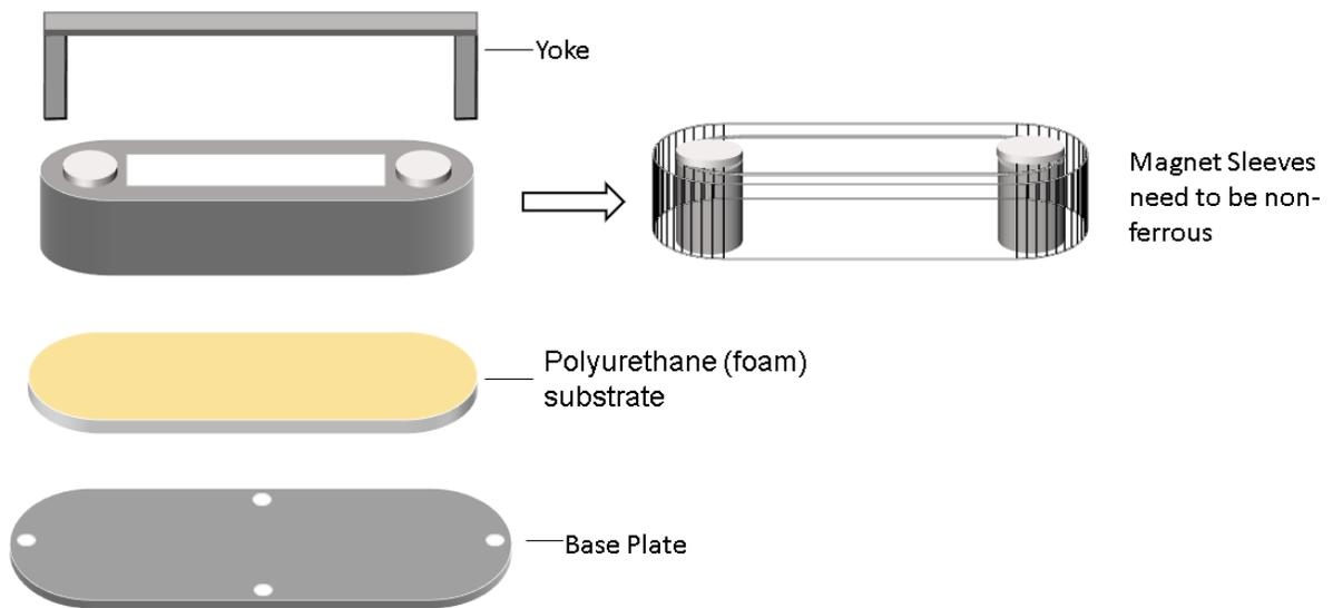
**Figure 5: Early layout of bobbin components.**
