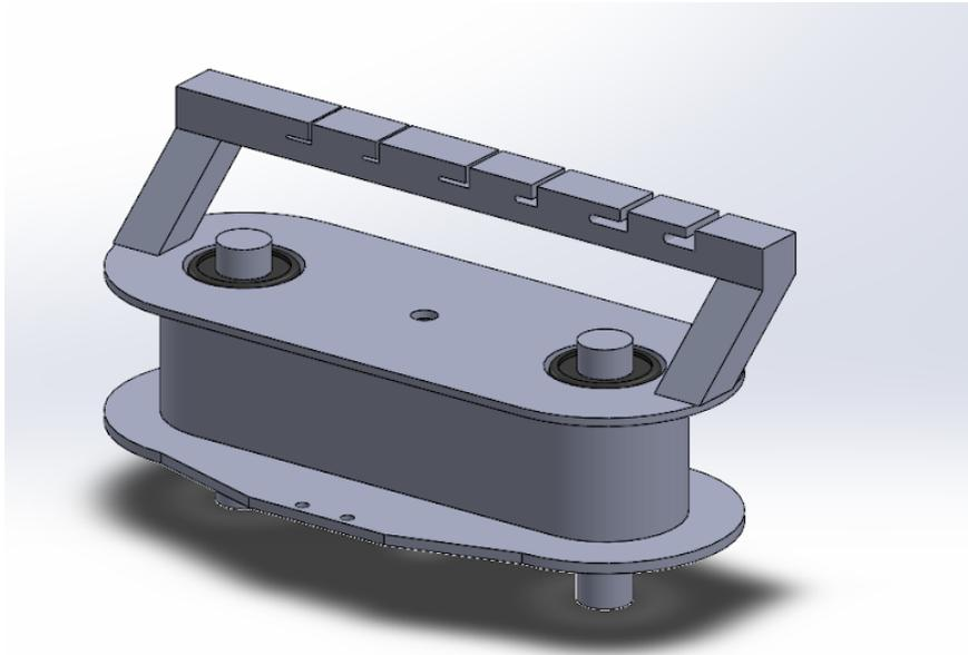
**Figure 6: Bobbin design with string-specific notches on yoke, hole for coil winder shaft, and holes for the coil leads.**
