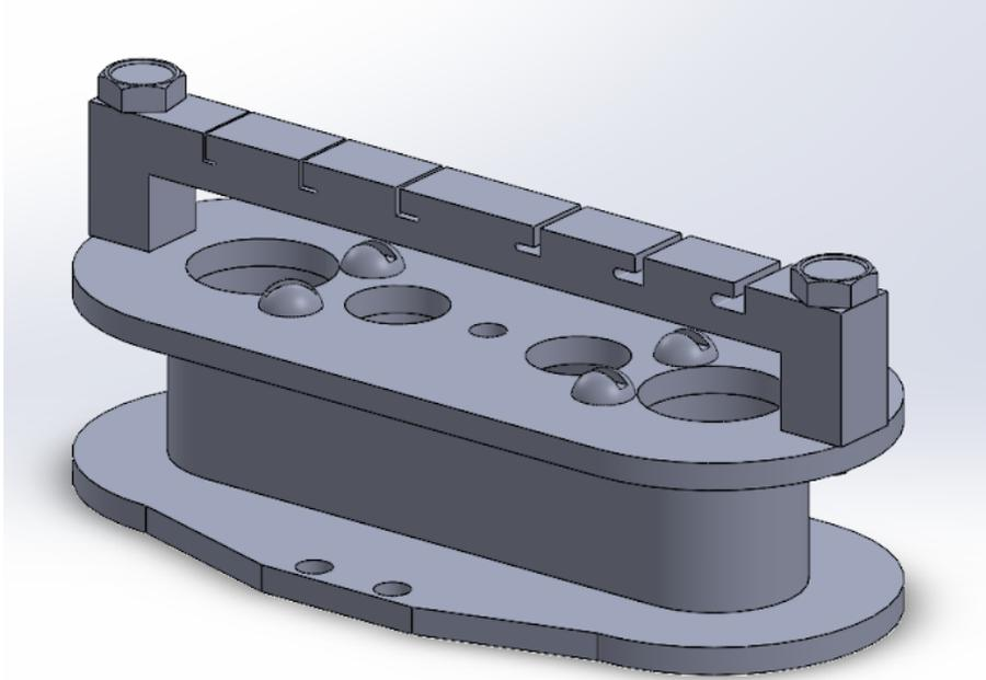
**Figure 15: 3D model of final yoke-bobbin assembly.**
