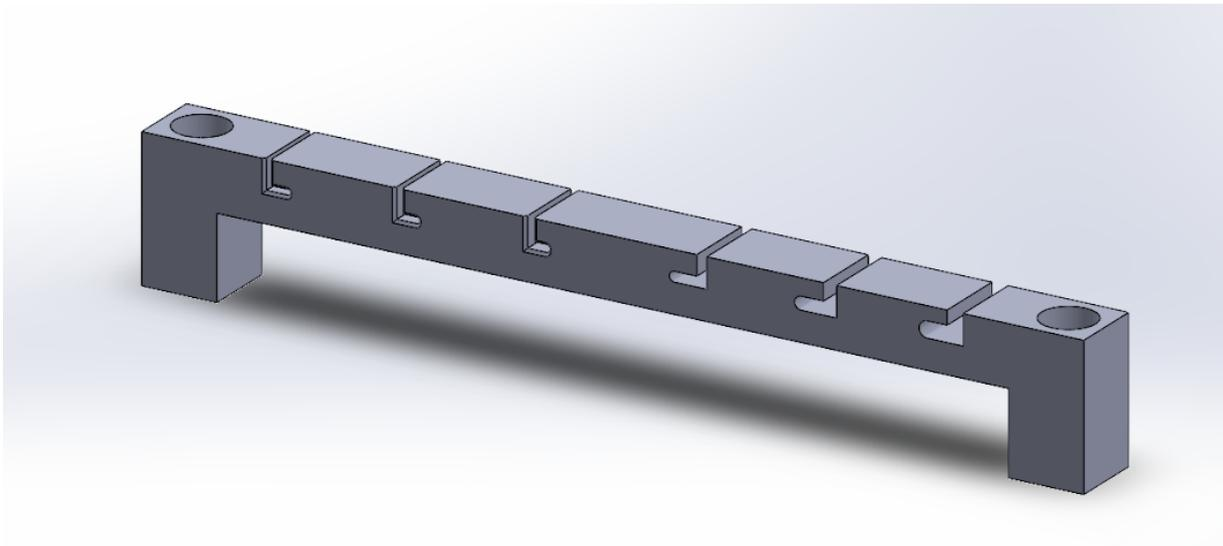
**Figure 28: 3D model of yoke with chamfers.**
